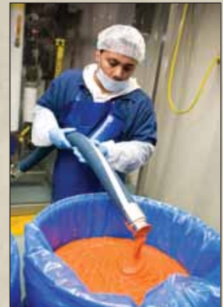
Left, trailer-lift system for unloading fresh carrots. Right, pureed carrots, that have been sanitized, chopped and pasteurized, are filled into drums in the HEP ® -filtered clean room.
