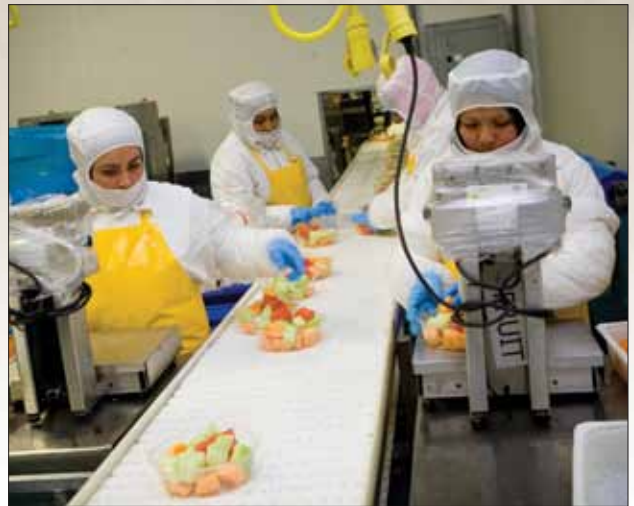
Fruit trays are being assembled and check-weighed within high-care facility before going to separate packaging area.
