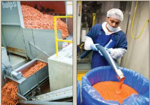
Left, trailer-lift system for unloading fresh carrots. Right, pureed carrots, that have been sanitized, chopped and pasteurized, are filled into drums in the HEP ® -filtered clean room.
