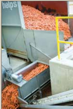
Left, trailer-lift system for unloading fresh carrots. Right, pureed carrots, that have been sanitized, chopped and pasteurized, are filled into drums in the HEP ® -filtered clean room.
